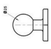
The device will be attached to a 1 inch ball head as shown in the picture above. This ball mount must be attached to the vehicle with tight screws at a location as described above. The diameter of the screw holes is 6.5mm and the distance between the holes is 40mm. When mounting on the dashboard, a support plate must be attached to the back to prevent the screws from breaking through the plate in the event of an accident to prevent the holder from flying around freely in the vehicle.
